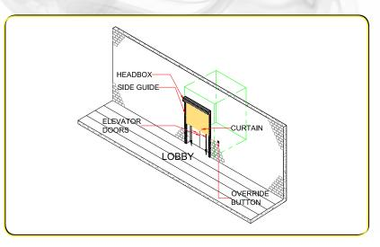
the elevator door, rendering the curtain invisible when retracted. Once deployed it permits a greatly reduced level of smoke leakage falling inside the international leakage requirements.
