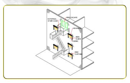
protection to the stairs from smoke, irradiance of heat and high temperatures as well as naked flames.
