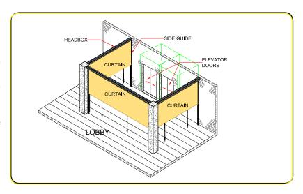
curtains. Again, when not in use there is no physical impediment or restriction but once required a full integrity and, if required, smoke sealed lobby can be created.
