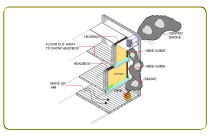
the perimeter edge. Sophisticated control systems allow for the curtains to facilitate these strategies by employing staged and separate deployments, level by level or even curtain by curtain, with multiple alarm inputs being reacted to.
